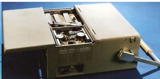
Fig. 5b. SPS for the Neurolab-B instrument https://rait-aerospace.com/photogalery/_018.jpg
